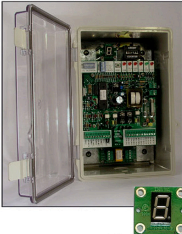
Includes Enclosure, "Gallons" Display and Credit Counter
